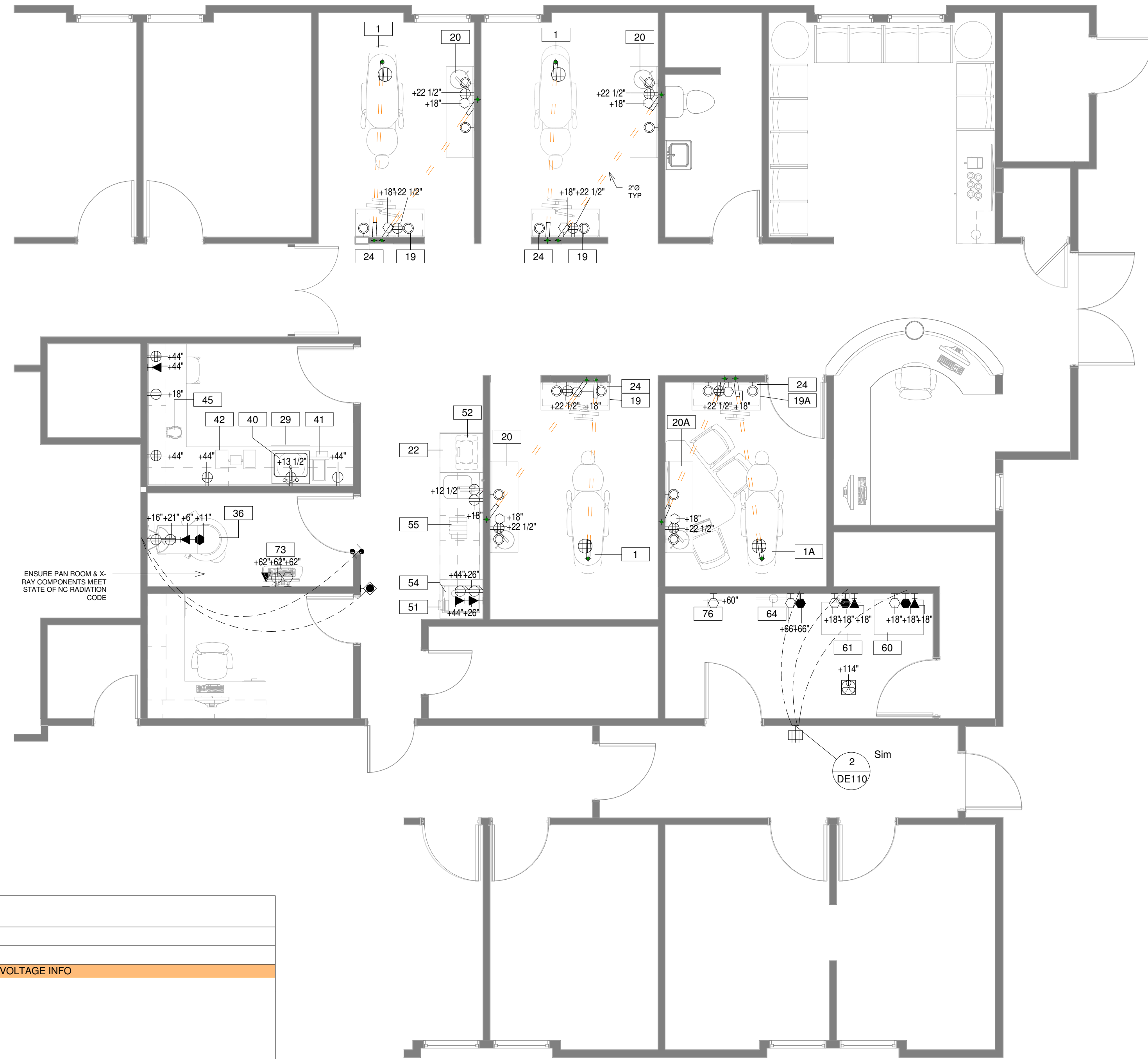
① LVL 1 POWER & LOW VOLTAGE PLAN 1/4" = 1'-0"
