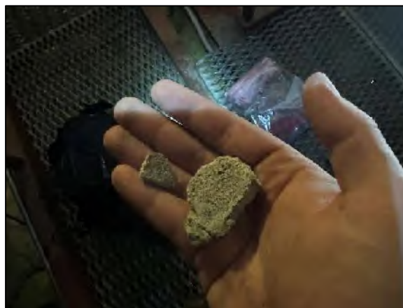
PHOTO 6 Close-up view of Sample BB-3 Central Wing - Attic 2% Chrysotile
